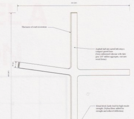
Figure 6. Diagram of one asphalt intersection part. Asphalt is set into a mesh earth grid above a compacted gravel base. Asphalt is rolled to solidify the hot aggregate mixture, creating a smooth street surface. Paving marking is rolled or stenciled directly onto the asphalt once it is set. Model built at one three-hundredth real size.
